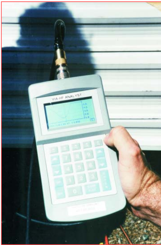
Testing the SGC with the AEA antenna scope, showing good tune on 40 meters with the AEA portable analyst.
